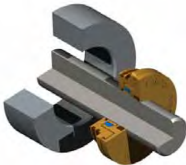
Figure 20 — Seal installation on Shaft
